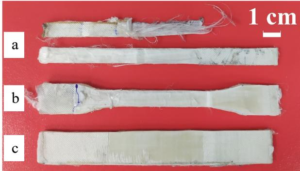
**Fig. 7.** Specimens after tensile testing: straight-sided (a), width-tapered (b) and large cross section (c).
